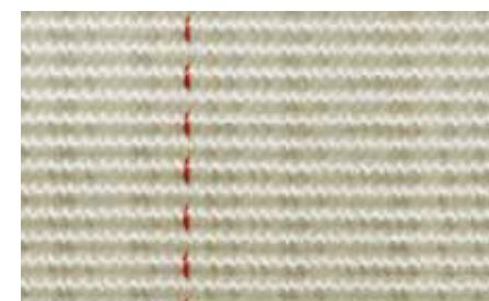
FLUITEX® E 1200 1.71psi@22ft3/ft2/min Thickness: 0.15", 0.19", 0.24", 0.31" Red tracer thread
